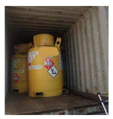
Routine container inspections show a high degree of non-compliance with declared DG containers including an excessive incidence of poor stowage and securing.
